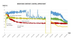
Figure 3: Registered moisture content for centre, upper part until 06.08.2018
